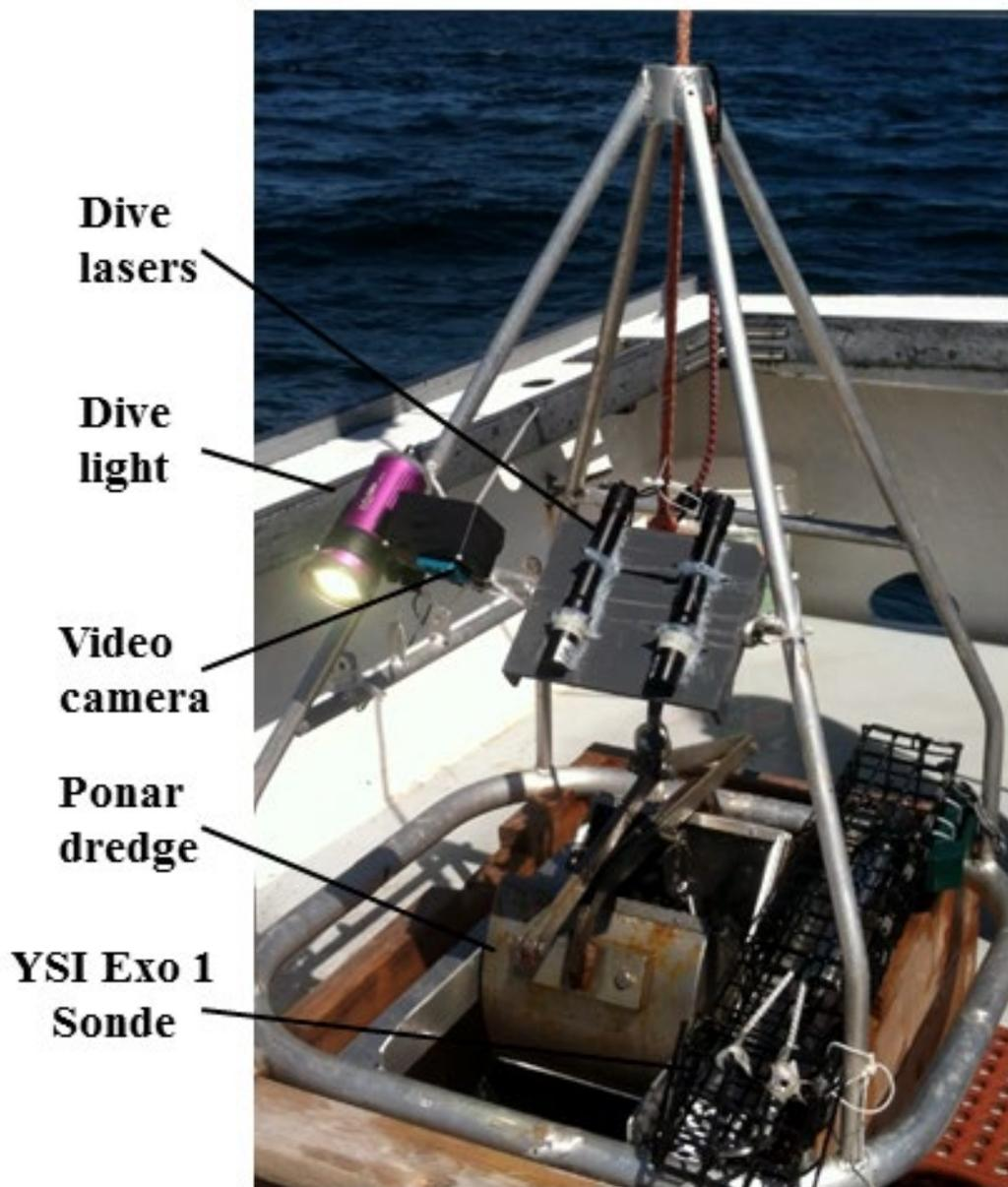
Figure 4. MCMI grab sampling platform. This sampling platform was used throughout the 2015 and 2016 field seasons.
